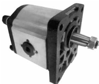
Group 2 - conical 1:8, European cover (Ø 36.5 mm), flanged connections
